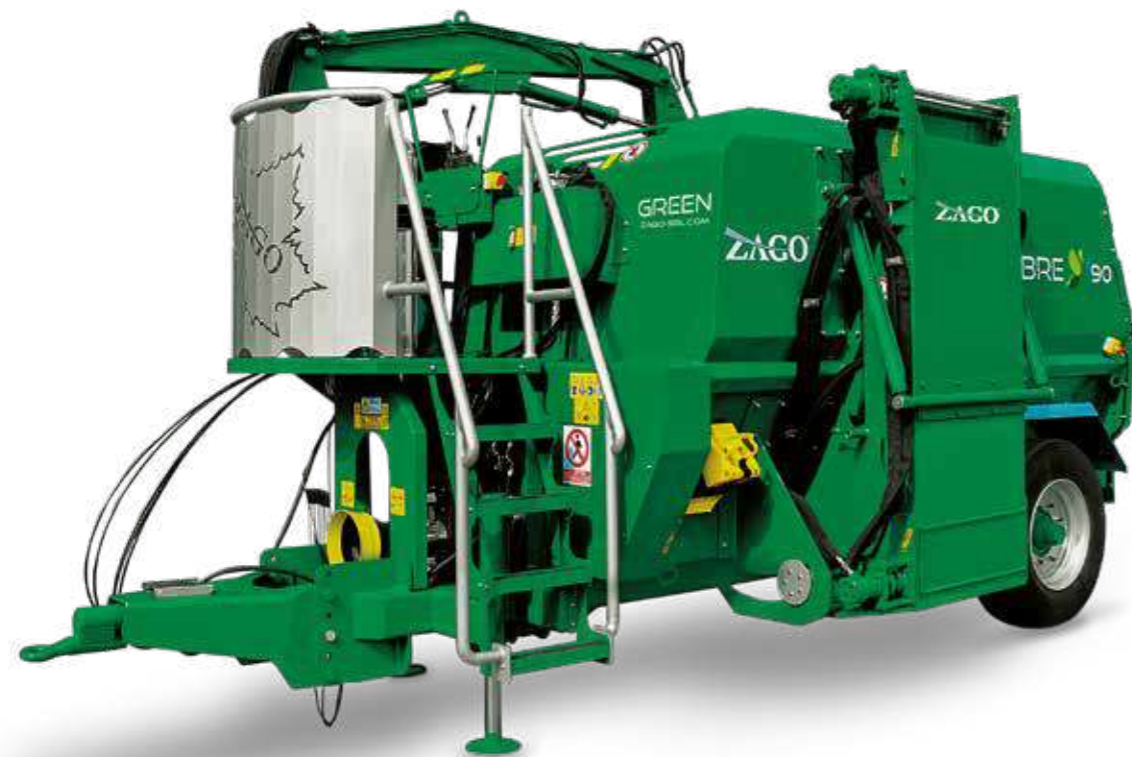
Eko Sabre 90 trailer with 2 augers and 2 m discharge conveyor
