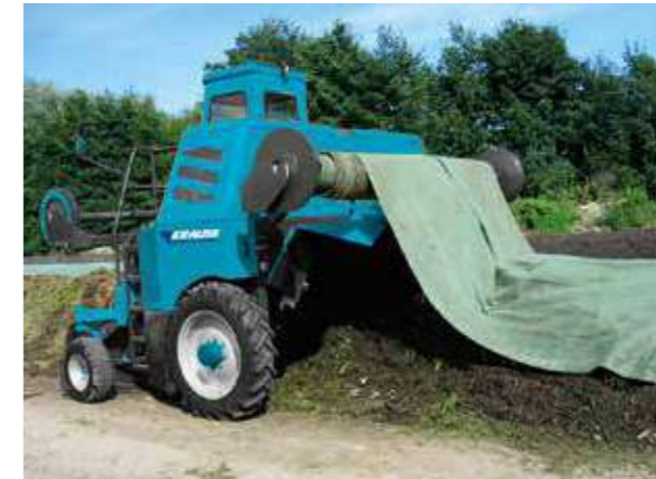
Compost cover roll-up and unrolling systems are available on all models.
