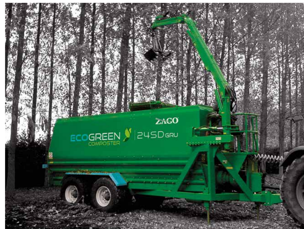
Ecogreen Composter 24 m 3 trailer with PTO drive and lateral loading crane
